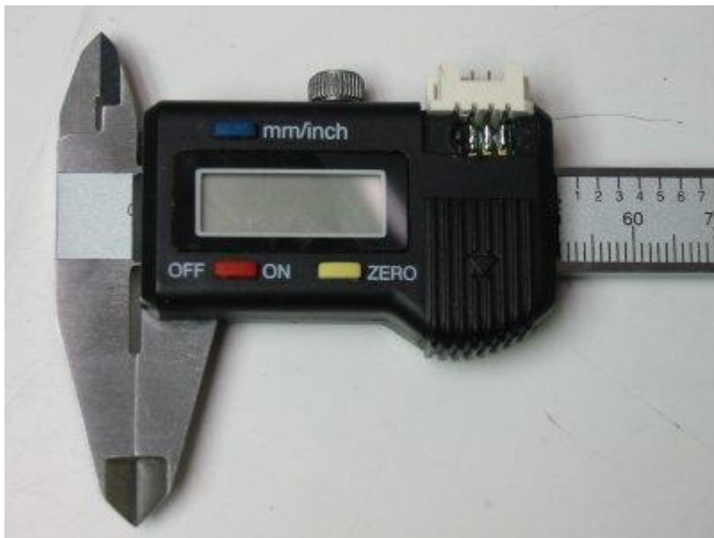
Connector soldered to caliper PCB - 2.0mm Hirose DF-3 series SMT right angle - DigiKey H2129-ND
