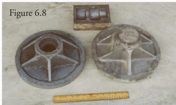
← The pattern (right), core box (top), and casting (left) for the bearing case
