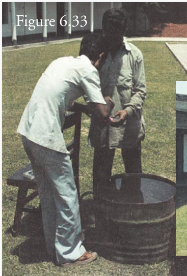
← In the first test, the die was immersed in a half drum of water.
