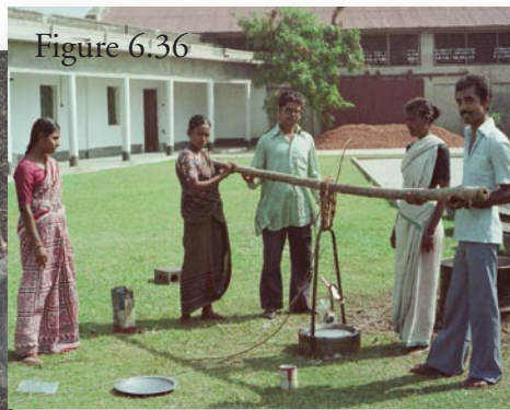
↑ Ready for another test using a full drum of water, which is half buried in the ground. The explosive is positioned above the blank.
