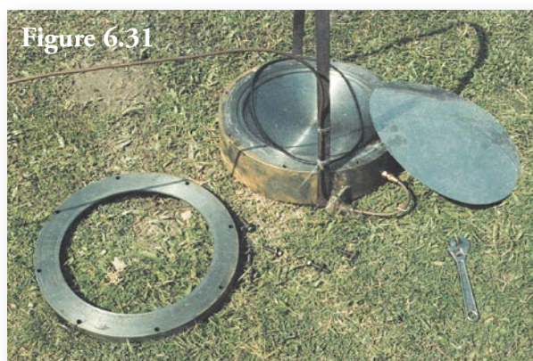
↑ The die used in explosive forming of the displacer dome. The stainless steel blank will be clamped to the die with an O-ring seal to make it airtight.
