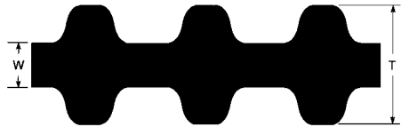
Fig. 37 Twin Power Belt Tolerances
