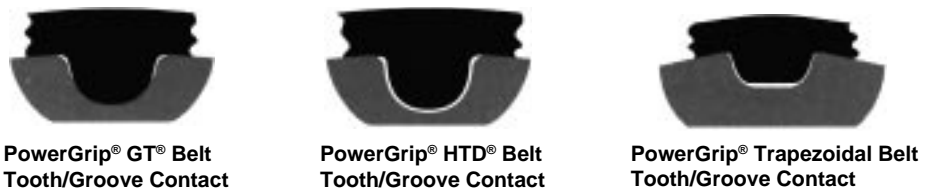
Fig. 3 Comparison of Different Tooth Profiles
