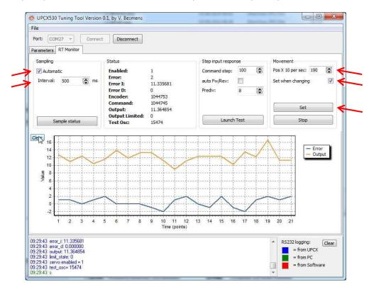
If you stop the motor shaft a little by hand, the positioning error will increase a little but the regulation will kick in and put it back to 0.
