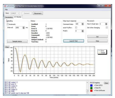
At some optimal point the result should look like this while the motor still holds its position well when its shaft is turned by hand and does not start vibrating again:
