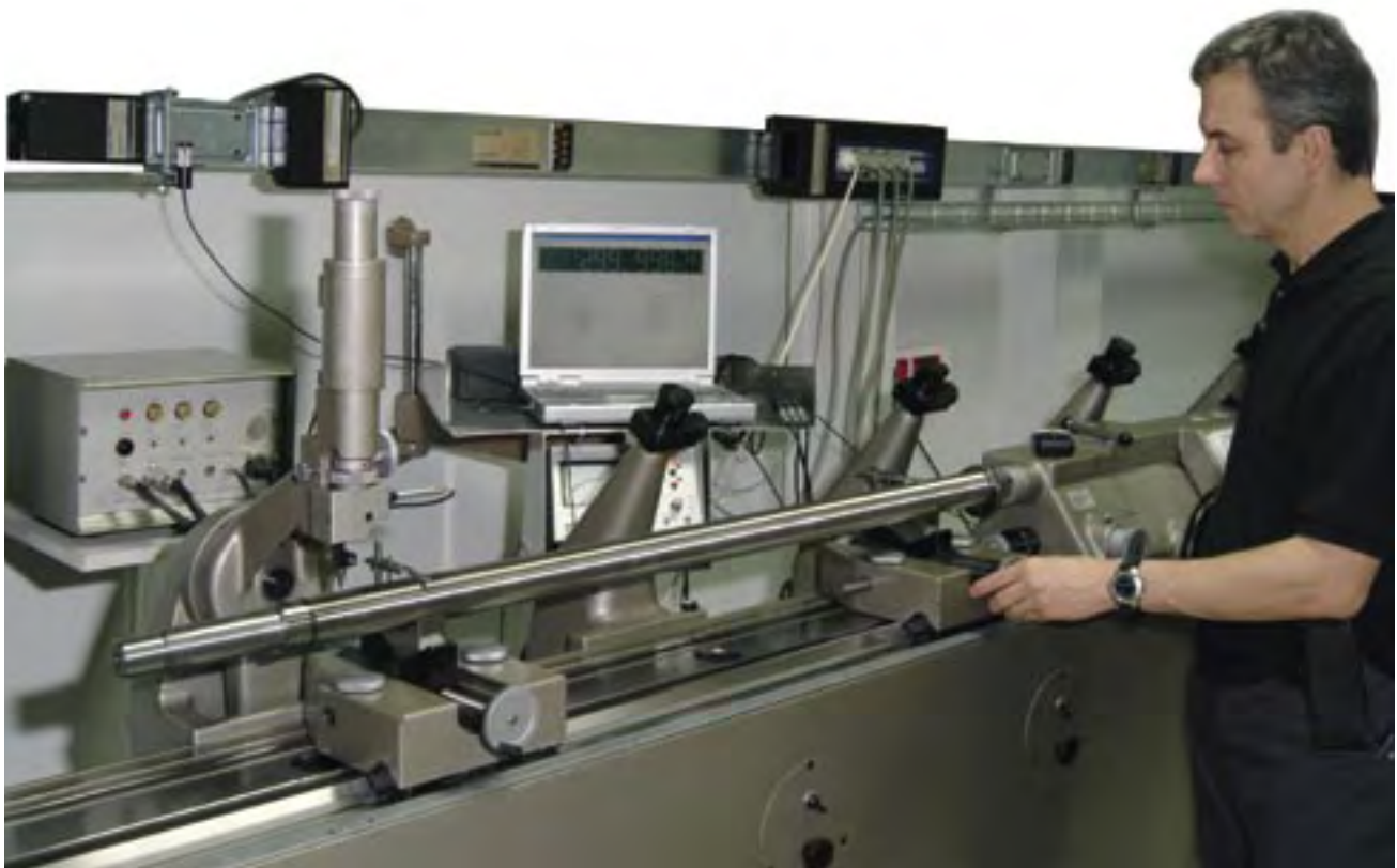
Lead error control interferometric test bench
