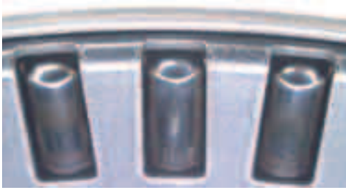
Photo 2. Improved contact type cage
