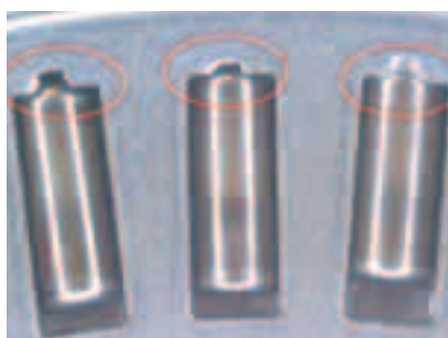
Photo 1. Wear of cage pockets (red circles)
