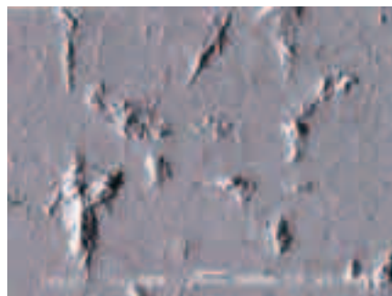
Photo 2 SEM image showing outer surface of tappet roller
