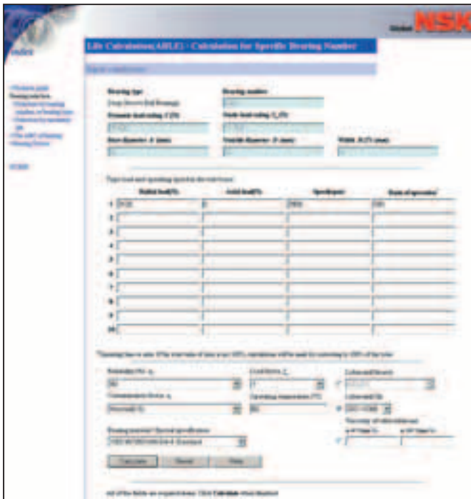
Fig. 6 NSK ABE Forecaster—Calculations for a selected bearing
