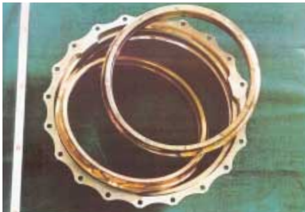
Photo 1 AP-treated bearing for aircraft gas turbine engines
