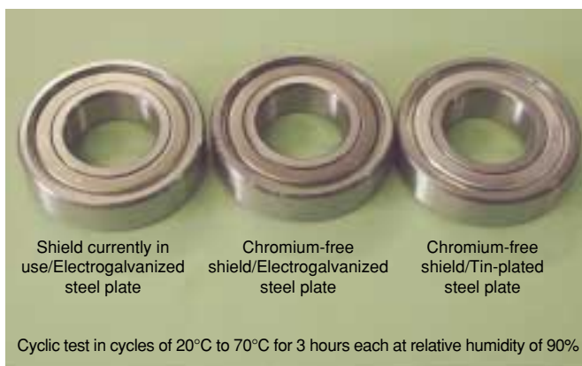
Photo 1 Bearing appearance after 1000 hours of shield rust testing
