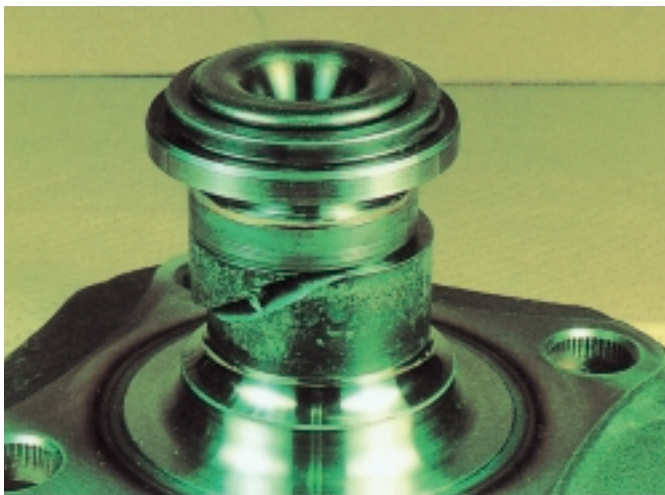
Photo 2 Condition of hub unit after static strength test (Swaged type)
