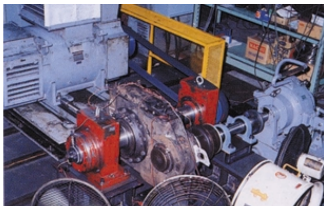
Photo 1 Full-size gear unit tester (0 Series bullet trains)
