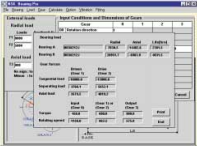
Fig. 7 Calculation results on bearings on a shaft with spur and helical gears
