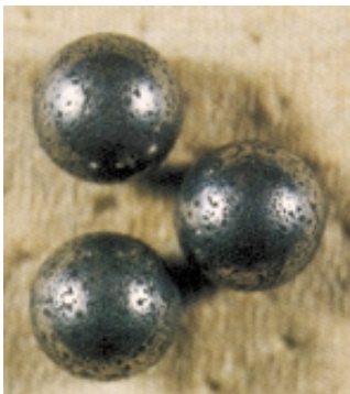
Photo 7 Balls of Linear Guide 1 (no K1 Seals)
