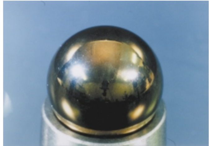
Photo 1 Tested ball (with AP treatment)
