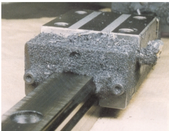
Photo 3 Linear guide after 2 000 km of operation while exposed to cast iron dust
