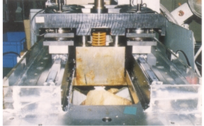
Photo 9 Endurance test simulating a food processing machine (water-immersion test)
