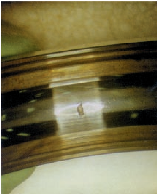
Photo 1 Outer ring flaking
