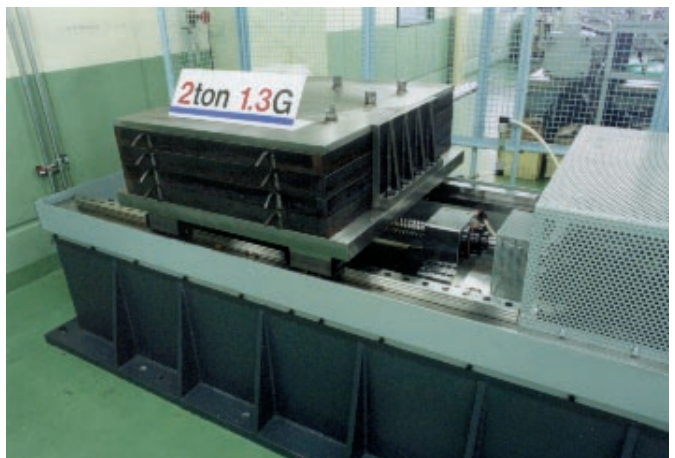
Photo 4 Endurance test of high-speed and high-acceleration/deceleration work table
