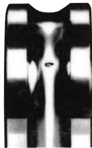
Fig. 5.1 Example of Flaking
