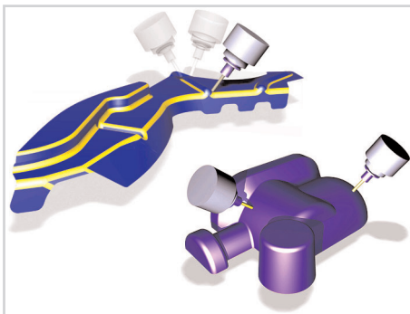
5-Achsen Simultan fräsen / 5 axis simultaneous milling
