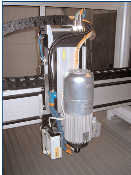
Kombination CONOPROBE-Laser und MAW 2.22-K - Spindelmotor / combination of CONOPROBE laser and MAW 2.22-K - spindle motor
