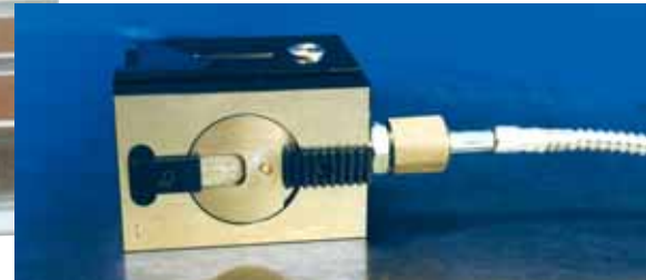
Underside of hydraulic clamp showing cartridge insert
