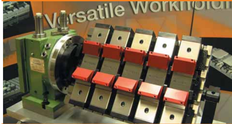
above: Hydraulic fixture for machining chain links in six operations below: 75-series trunnion on display at Mach'2002, Birmingham UK
