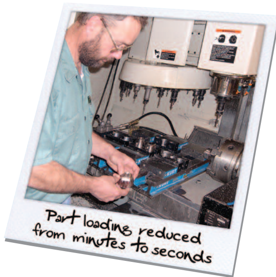
At 10,000 RPM and 240in/min we needed rigid workholding
