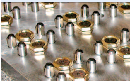
Solution: High density fixture clamping four parts per station.
