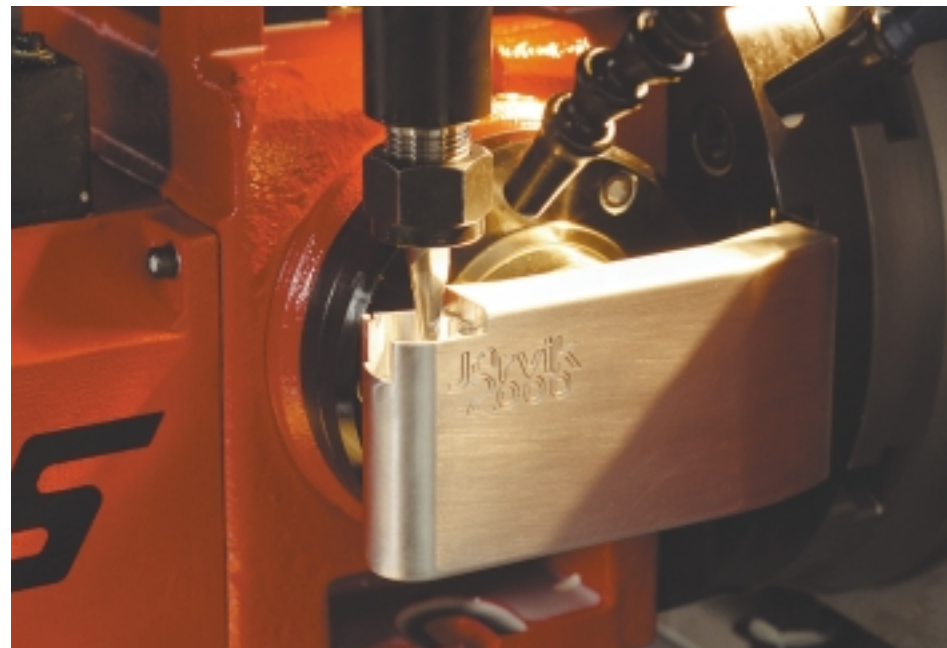
A version of the axial-flow blood pump being built at Jarvik Heart in Manhattan uses external batteries and electronics. The control boxes (above) and other components are machined on a VF-1 with a T5C tilting rotary table.
