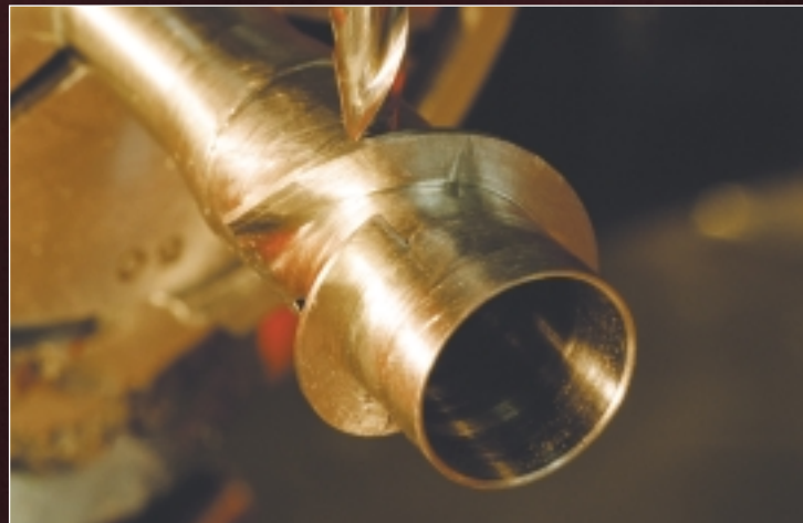
Above: Cutting the contour-bladed impeller. Below left: A three-arched inflow bearing support, a machined impeller and an outflow elbow and bearing support.
