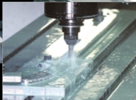
The 50"x20"x25" travels of Stamco's Haas VF-4 allows them to machine runners for Pierre Lueders' bobsleds without refixturing.
