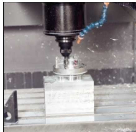
Multiple fixtures are used when machining many of the 50-plus parts used in the Aurora V-8 oil pump. Perfection is a must.
