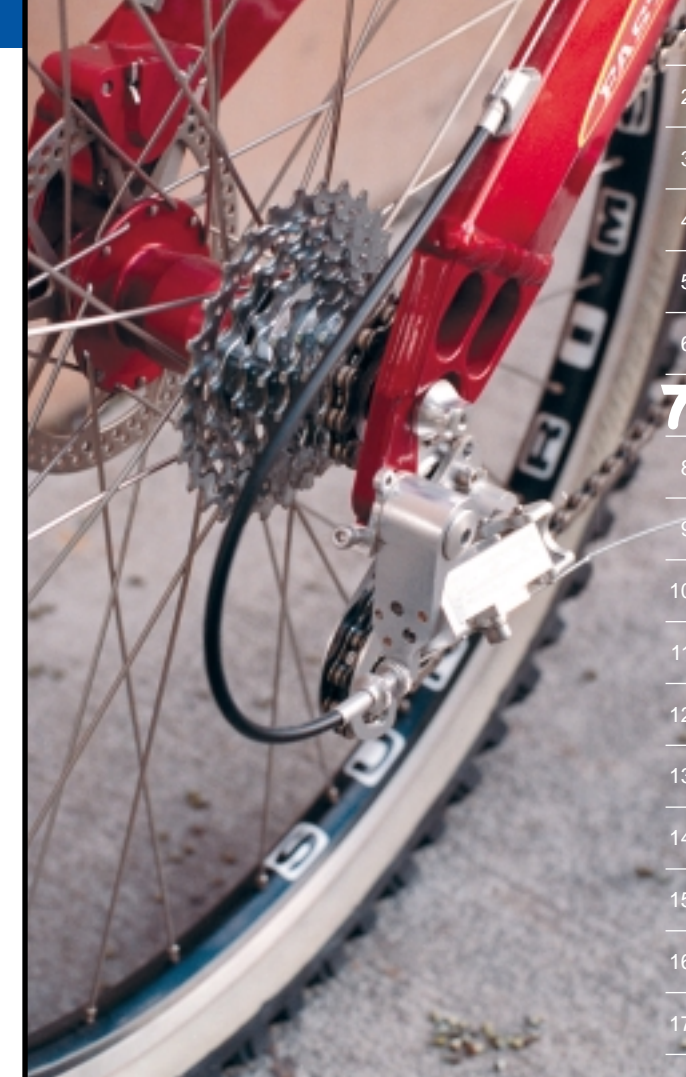
ProShift's derailleur systems are completely user serviceable with replacement parts available. Very important features for rough & tumble mountain bike enthusiasts.
