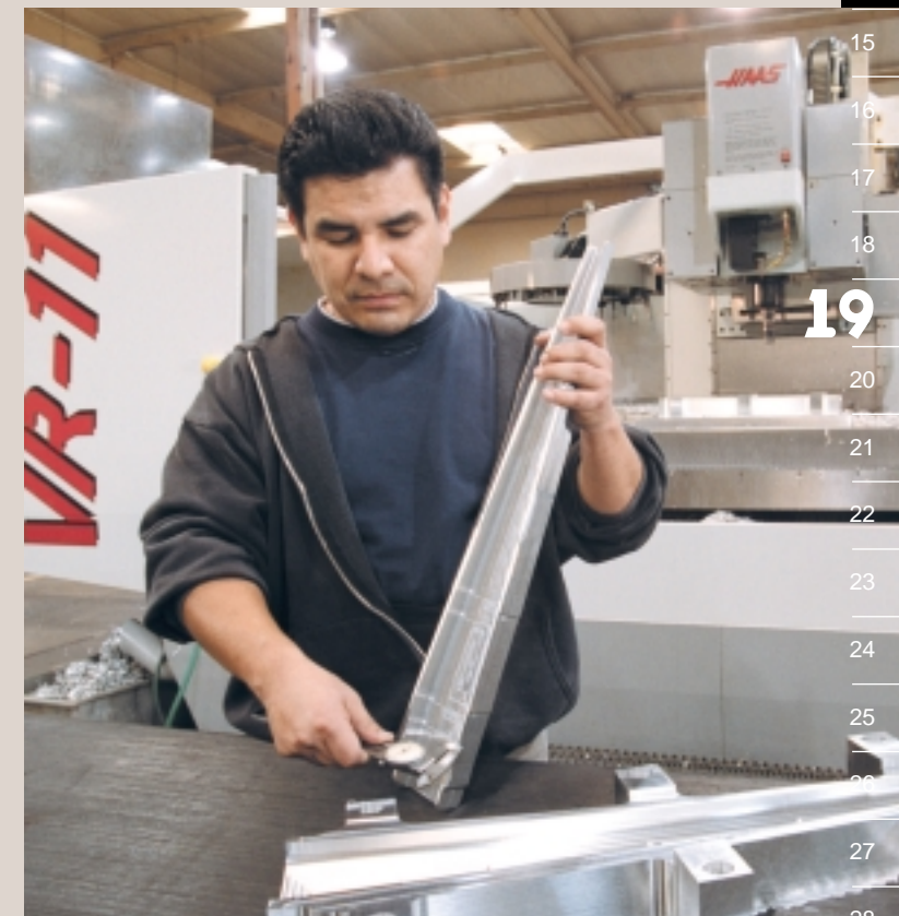
Frank Escobar checks a completed emergency escape hatch upper sill that was machined on one of Aircraft Engineering's three Haas VR-11s.
