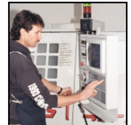
Gary Hickman at the control of the Haas lathe. Precision Billet has reduced programming time substantially with several control features unique to the Haas lathe, such as G81, G83 and G84 canned drilling cycles identical to those found on mill controls.
