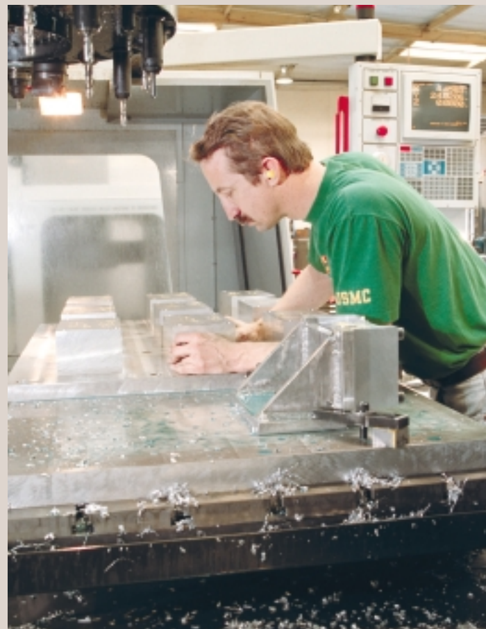
Hal Purdy sets up a Haas VF-6 to machine emergency escape hatch brackets. The large table of the machine allows Aircraft Engineering to machine nine pieces at a time for high productivity.
