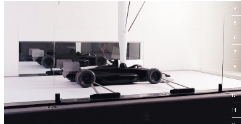
By using a precise scale model sized at 45-percent of the full-size car, Swift uses its wind tunnel to check the aerodynamic forces generated by different body panel modifications.
