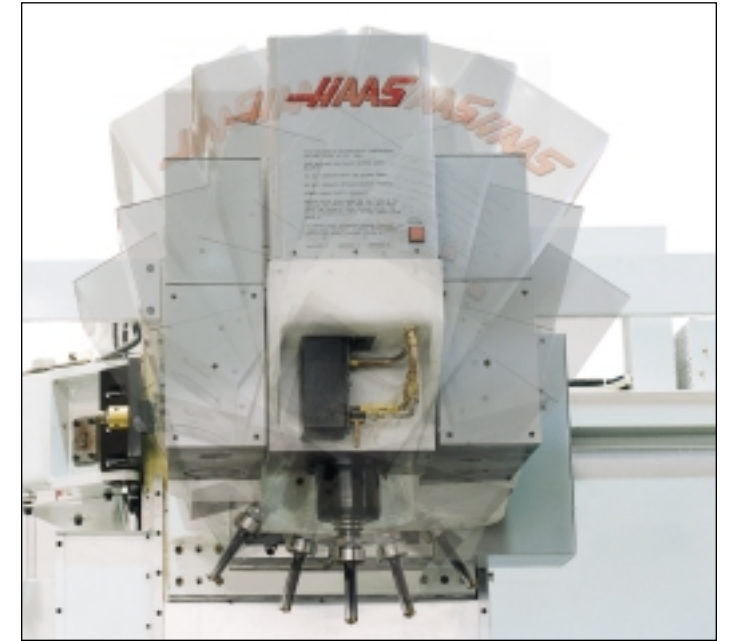
The five-axis spindle head of the new VR-11 provides an incredible \pm 32 degrees of rotation on the A and B axes, as well as rotational feedrates of up to 250 degrees per minute.
