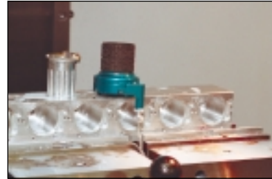
Computer-designed and machined out of 6061 T-6 aluminum, the Protwist Shifters replace factory plastic.
