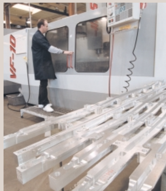
The travels of the Haas VF-10 allow Aircraft Engineering to machine long parts like these 82-inch-long stringer splices with ease. Steve Larabee monitors the process in the background.
