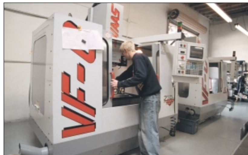
The Precision Billet crew can load ten tool offsets on the Haas VF-Os in the same time it took to load two tool offsets in the previous machines.
