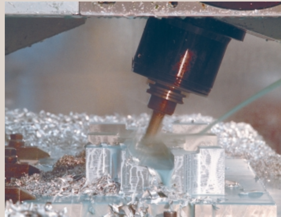
Aircraft Engineering uses their Haas VR-11s to machine 5-axis parts like this emergency escape hatch part in fewer setups.
