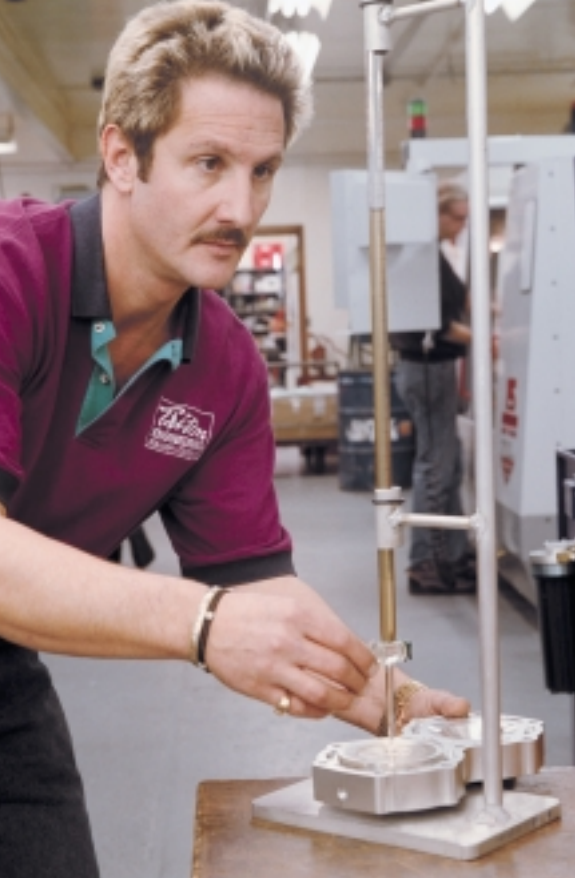
Ron Gitlin measures the combustion chamber volume of a Yamaha twin watercraft cylinder head. Heads are machined on a Haas VF-3.
