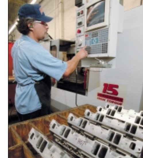
Roy Salas sets up a cylinder head finish operation on a Haas VF-3.
