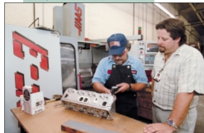
Scott Herrmann, right, looks on as Roy Salas checks the accuracy of valve-guide holes in a small-block Chevy cylinder head. Many of the finish operations are performed on Haas VMC's.
