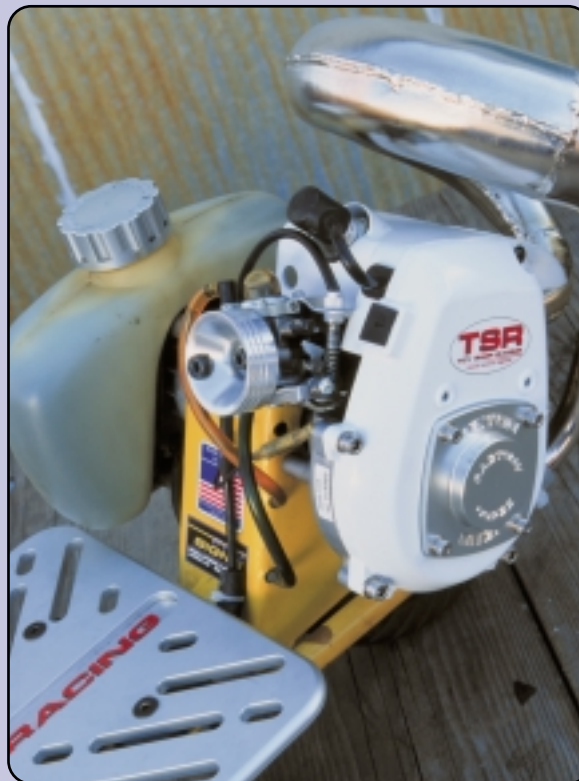
The monstrous 22.5 cc Go-Ped power plant, complete with Triton parts.
