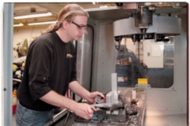
David Weaver sets up to machine a water rail for a Yamaha 700 triple snowmobile.
