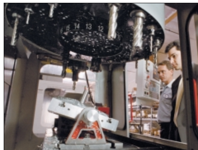
Danny Hennig, left, and Michael Allawos check a 4th-axis set up for an aluminum rib assembly Mikana manufactures for McDonnell Douglas.
