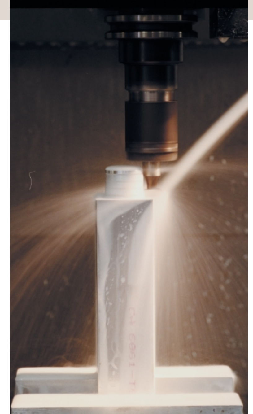
Machining of a water rail for a Yamaha triple snowmobile.
