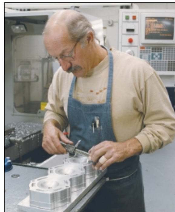
Wayne Sturm measures the combustion chambers of a Yamaha triple cylinder head machined on Triton's Haas VF-3.
