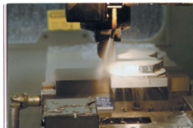
Triton burns the perimeters of their cylinder heads at 10,000 rpm and 130 ipm on a Haas VF-3 VMC.
