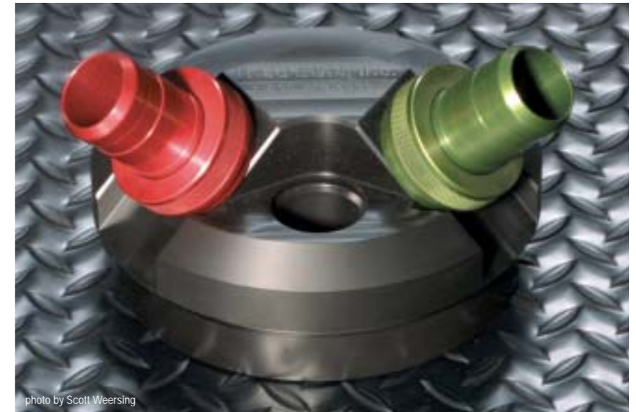
The top cover for an underwater breathing unit, above, is machined in a single setup on a Haas VF-2 using an HRT 160 rotary table mounted on an angle block. The setup is pictured below.
