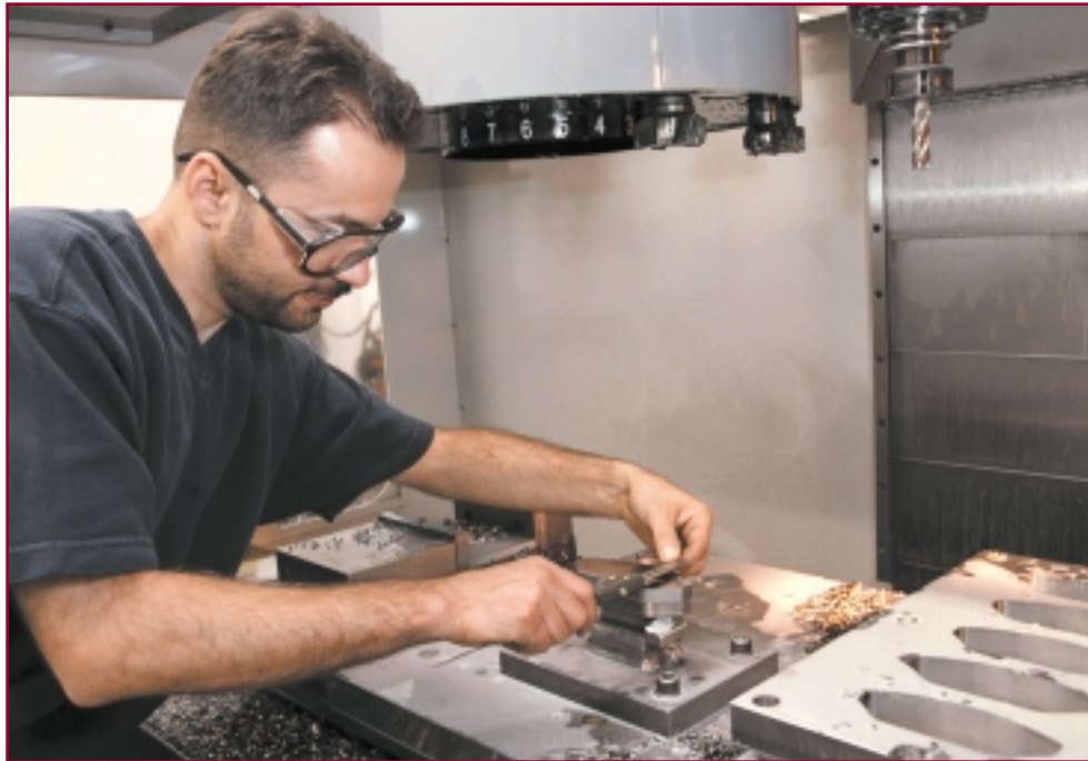
Nabil Khanania, above, checks the dimensions of a punch for a set of disc brake tooling. The matching cavity plate is shown at right on the machine.
