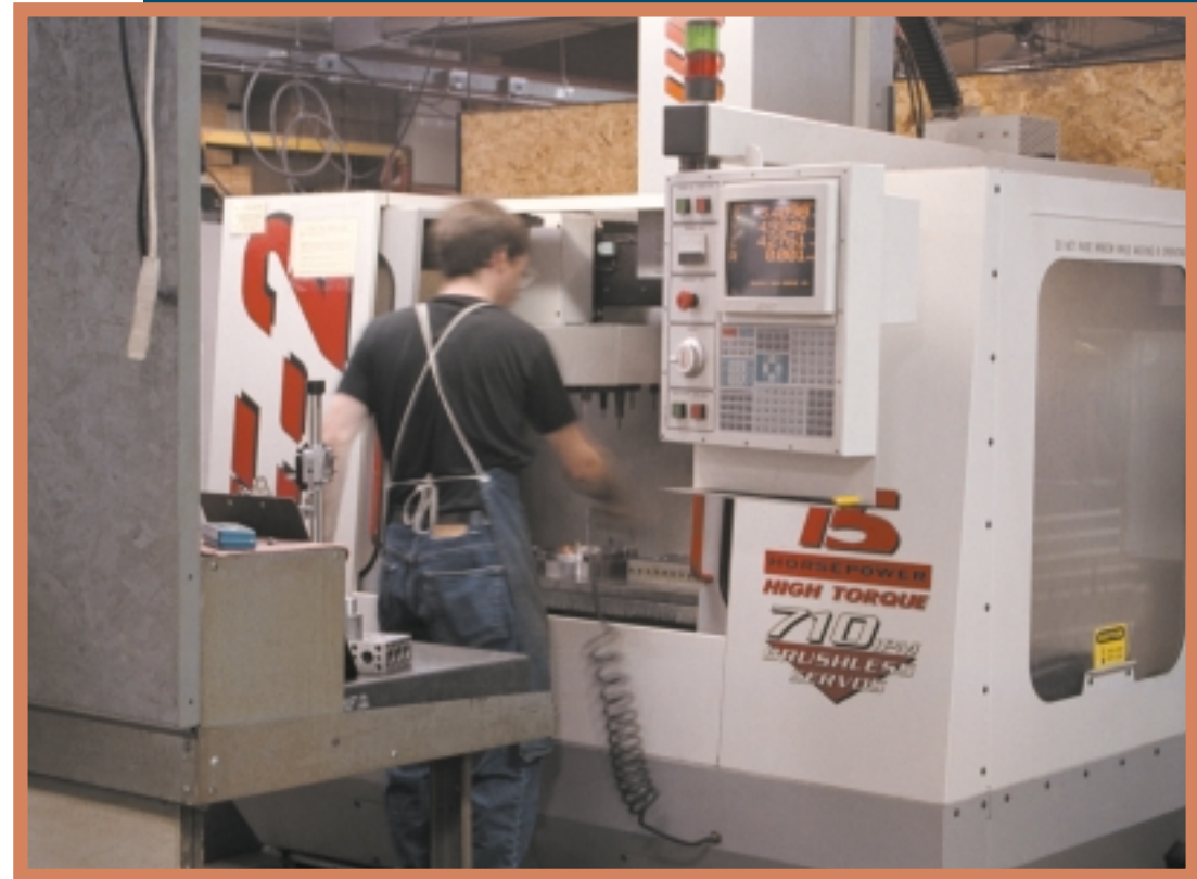
Long-term Ranger machinist Kirk G. Longuski produces first-rate fuel-pump reservoir screens on a Haas VF-2.
