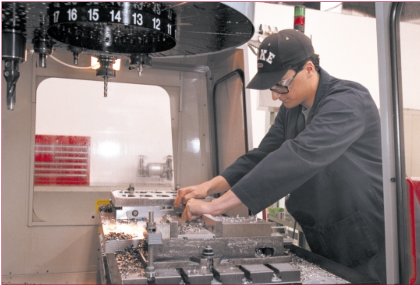
Dan Beaudin sets up to machine another punch out of 4140 HT alloy steel for a set of disc brake tooling.
