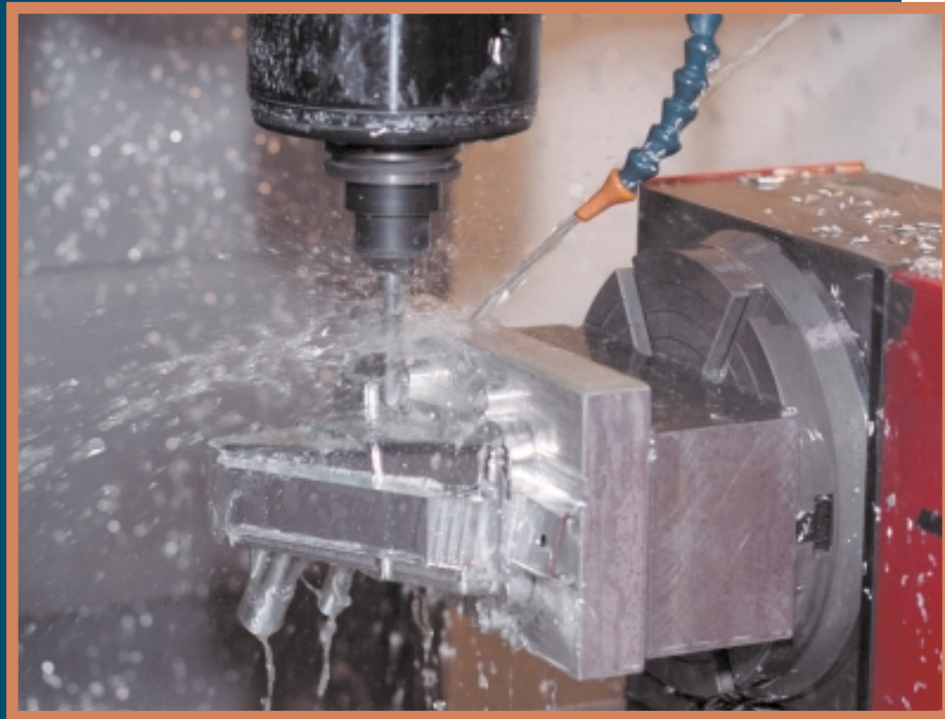
Many of the parts machined by Ranger are prototype components for steering systems. Above, a reservoir body for a power steering system is machined using a 4th-axis rotary table.
