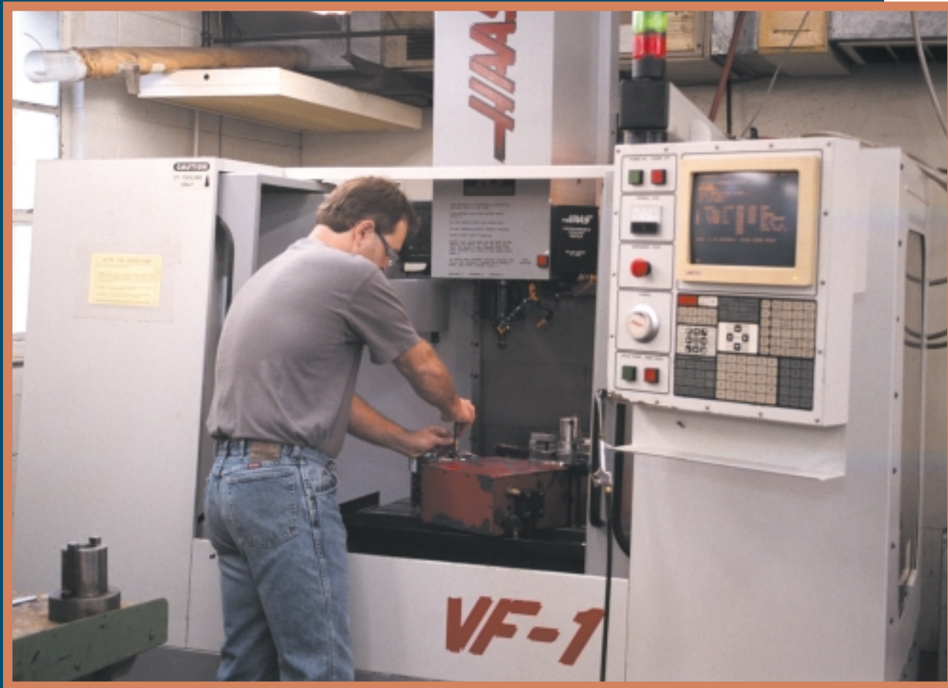
Tony Martin sets up a job on a VF-1 with 4th-axis rotary table. Many of the prototype parts Ranger produces require machining on multiple sides. Haas rotary tables help reduce the number of setups.
