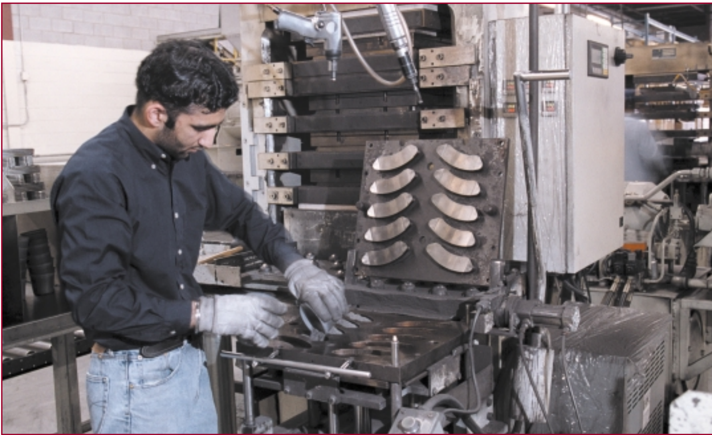
Rupinder Dhaliwal fills a set of disc brake tooling with a loose mixture of friction material before putting the tooling into a 400-ton curing press.
