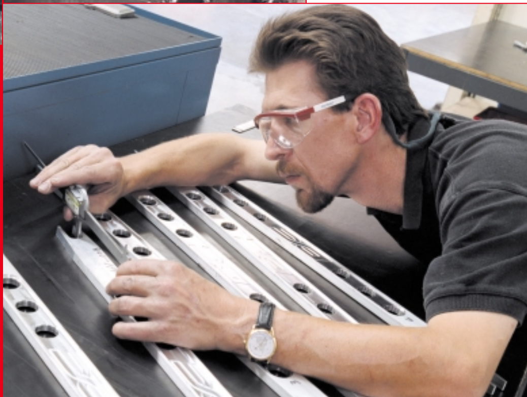
Kevin Young sets up suspension tie-bars for machining on a Haas VF-2, then inspects the finished parts as they come off the machine.
