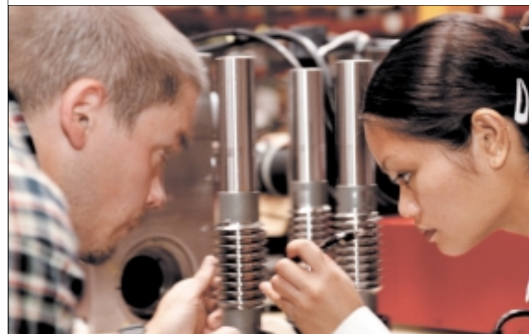
Mechanical engineer Andrew Harnett shows CSUN engineering student Helen Avila how to check for surface wear on a worm shaft.
