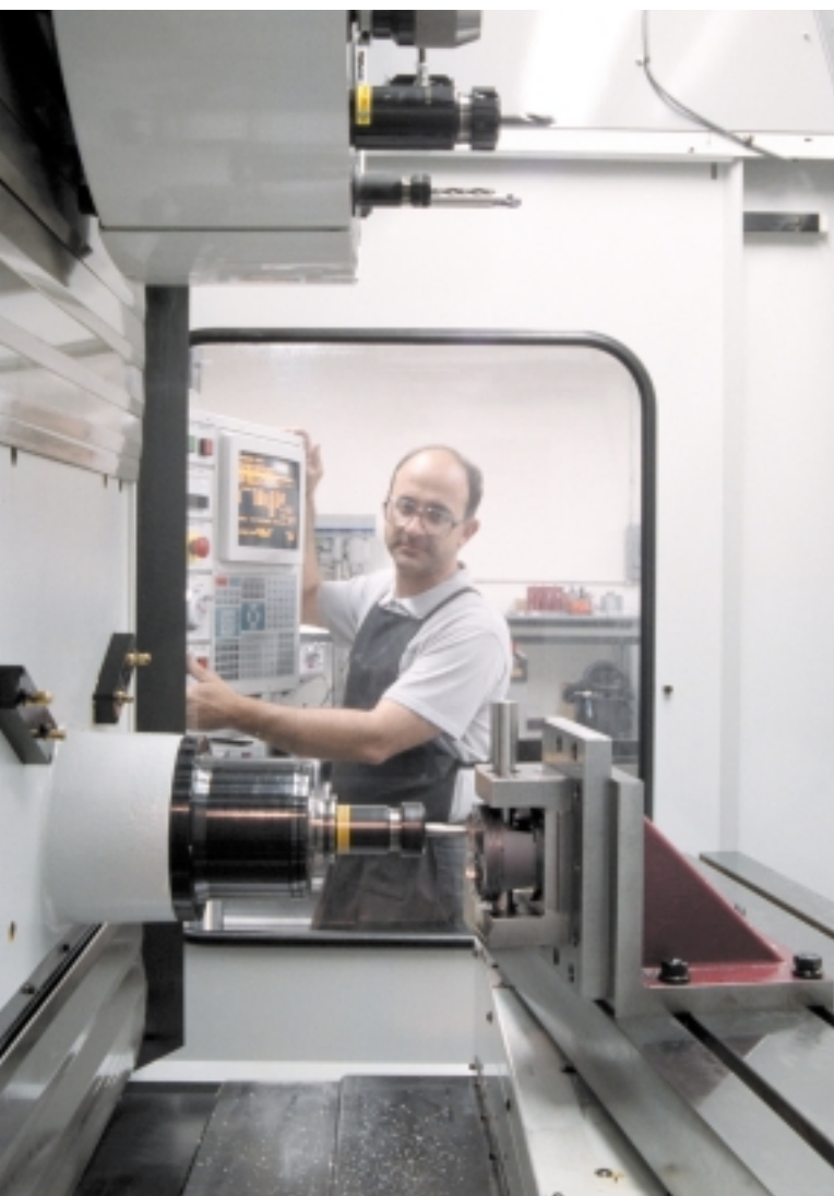
Many of the 4,000-plus parts used to build the Ilmor IC108-series racing engine are replaced at every rebuild. The majority, such as this piston being cut on the Haas HS-1R, are machined from raw or forged billets at the Ilmor facility.
