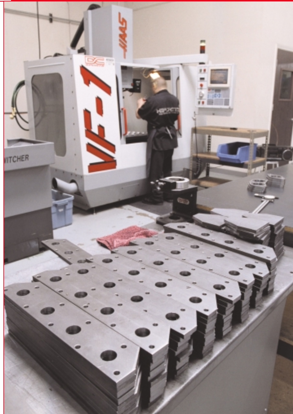
Header flanges are machined in two operations. First, the mounting holes and center of each exhaust port are drilled, then the mounting holes are used to fixture and locate the flanges as the outside profile is cut and the exhaust ports are interpolated to size.
