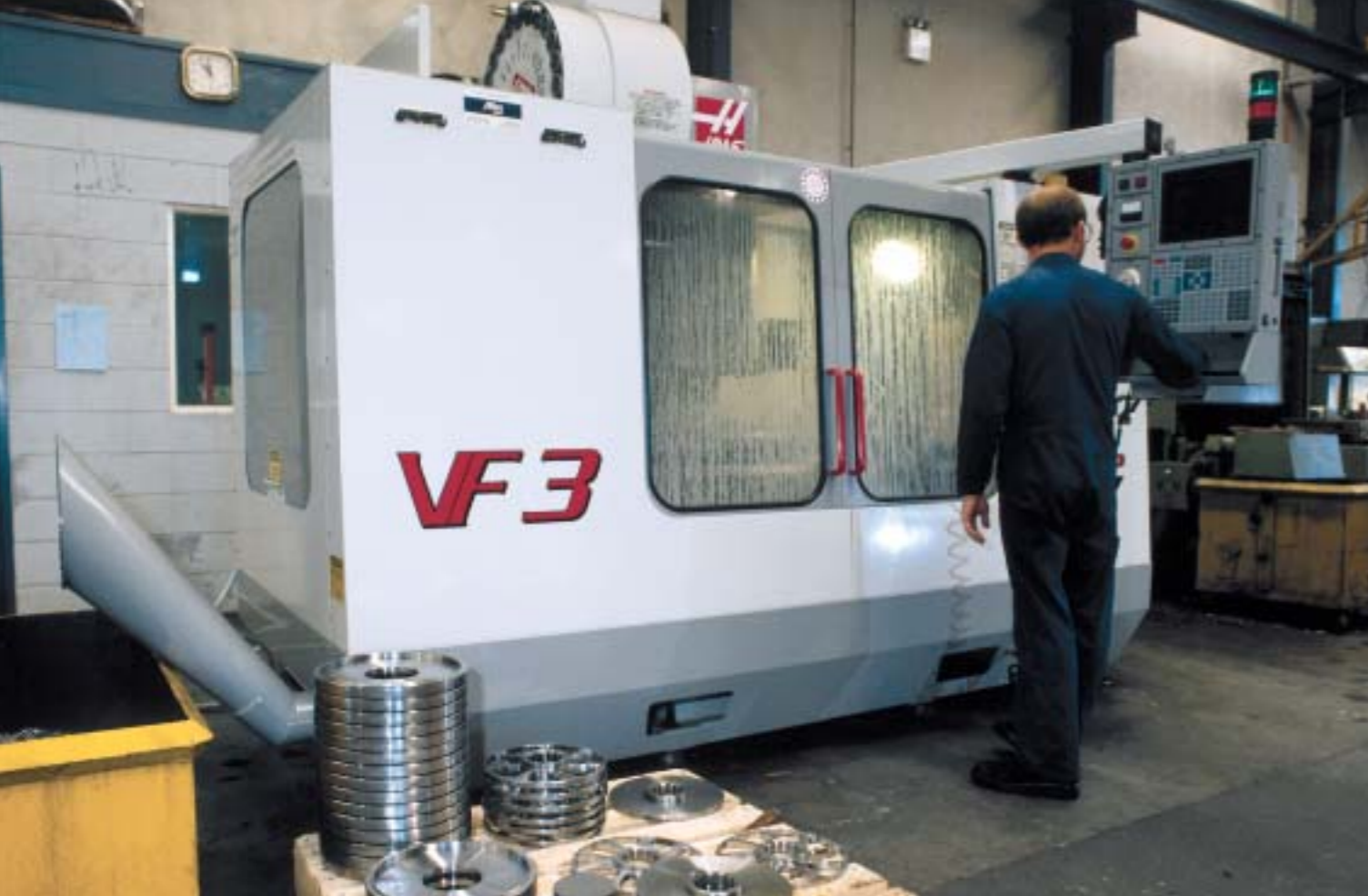
Above: Crown Engineering uses a Haas VF-3 to machine grinding disks out of D2 tool steel for a tyre recycling machine.
