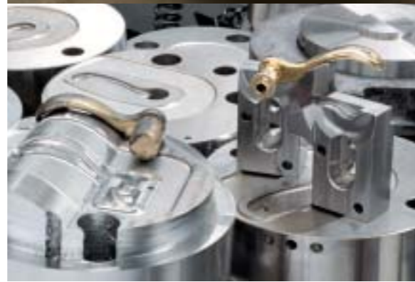
A set of forging dies and the artful handles they produce. Dies are cut out of H13 tool steel; finish cuts are taken after hardening.
