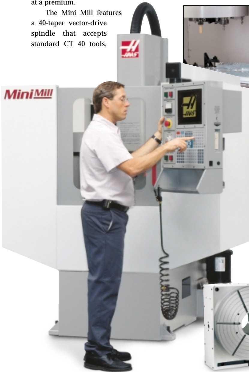
The Mini Mill's 40-taper spindle delivers 33 ft-lb of steel-cutting torque at 1,200 rpm, and spins to 6,000 rpm for finishing work. Combine that with travels of 16"x12"x10" and a 36"x12" table, and you have a small-footprint VMC that can easily handle the typical machine shop job.
