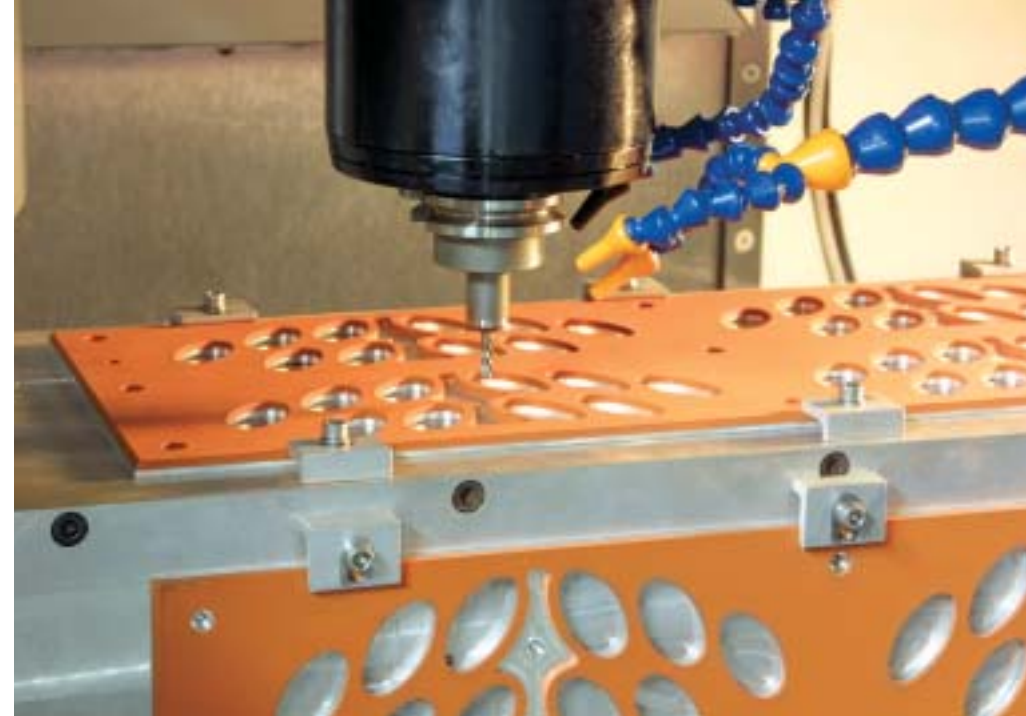
Using a Haas rotary table and a four-sided tombstone, Gemel Precision Tool Company reduced their cycle time for these parts from 45 minutes per plate to 4 minutes. The parts are machined on a Haas VF-3 equipped with a 15,000-rpm spindle and high-speed machining software.
