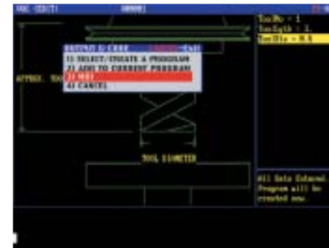
Once the information has been input, a pop-up menu prompts the user to select a location for the G-code output. In this case, MDI is selected.
