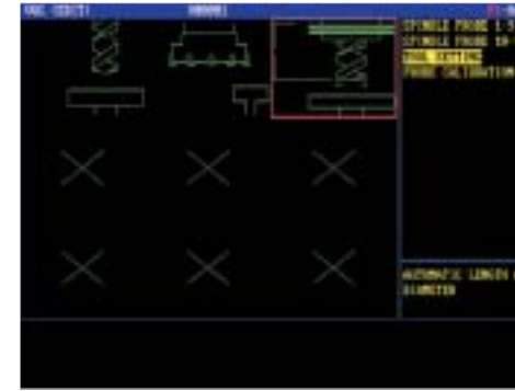
Select the Visual Quick Code template that represents the probing operation you want to perform. In this case, it's automatic length and diameter measurement.
