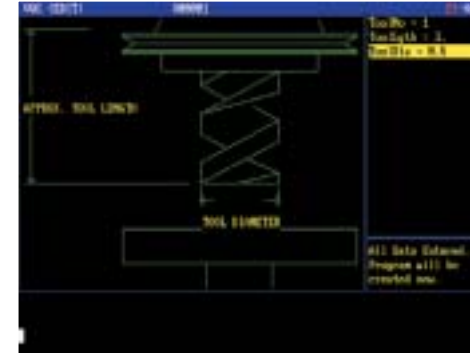
Fill in the basic information requested by Visual Quick Code: tool number, approximate tool length and approximate tool diameter.
