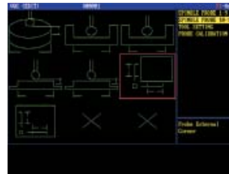
Select the Visual Quick Code template that represents the probing operation you want to perform. In this case, probe an external corner.
