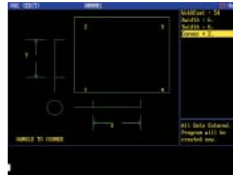
Fill in the basic information requested by Visual Quick Code: offset number (e.g., G54), approximate X part width, approximate Y part width and which corner to probe.
