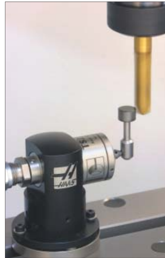
Once a probe routine to measure a tool is created using Visual Quick Code, tool length and diameter are measured automatically and the offsets are recorded in the Haas control.
