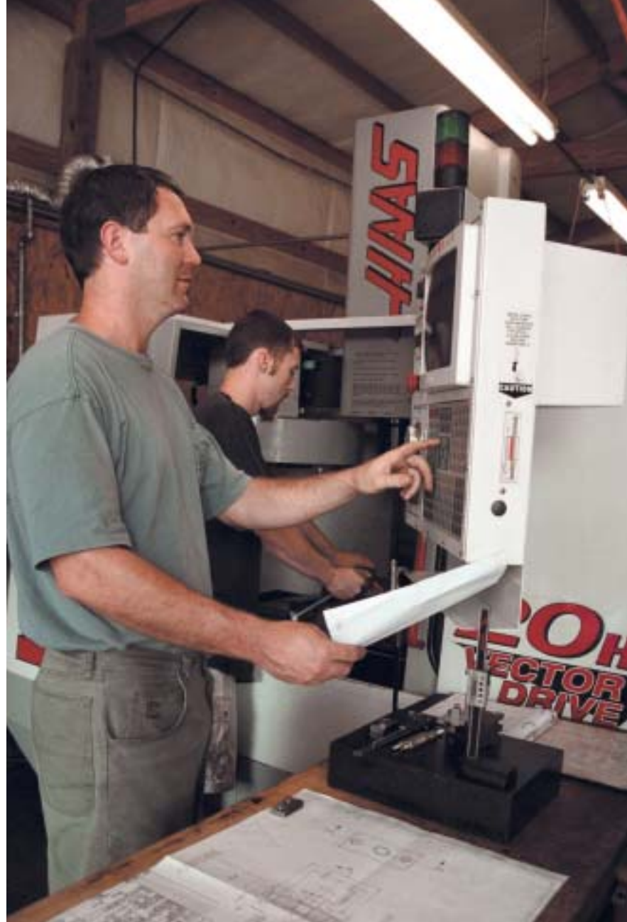
CNC programmer Jeff Mauney, front, programs the machine for the second operation on a part while operator Michael Lail changes over the setup.
