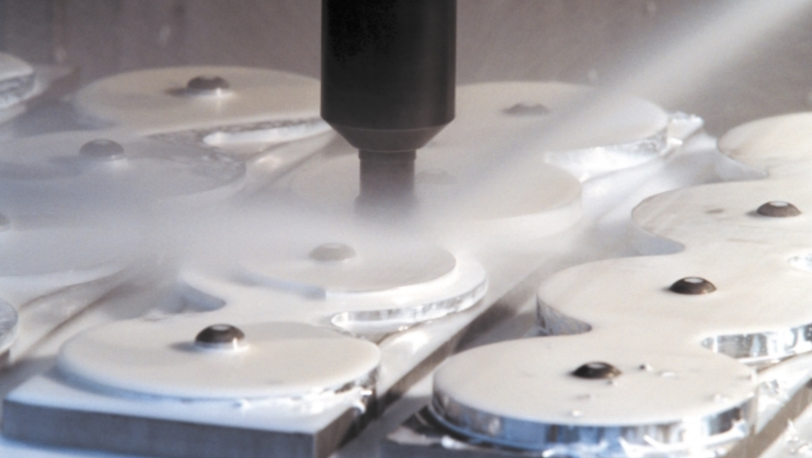
The major components of a Mathews bow, including the idler wheels (above) and risers (far right) are machined from aluminum billet. Multiple fixturing allows Mathews to get finished parts off the machines every time the doors open.
