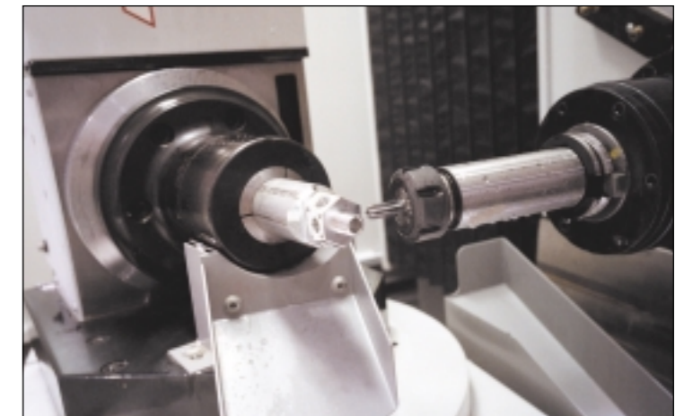
Lower left: The prototype HS-1 Auto Bar, a five-axis HMC with bar feed capabilities, also attracted much attention during the show.
