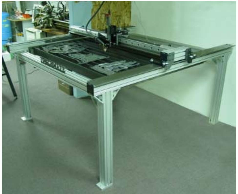
Above: Finished "bolt-together" Small Shop system, shown with Hypertherm manual plasma torch.
