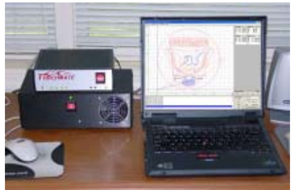
Torchmate electronics and software can be used with any IBM compatible laptop or desktop computer running on Windows 2000, Millennium, or XP (either version).
