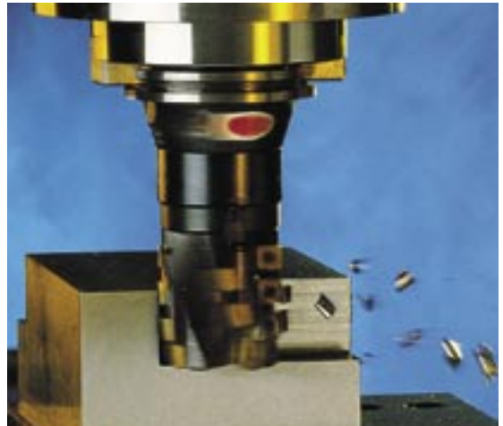
Power milling with Graflex Modular System: metal removal rate 432 cm 3 /min
