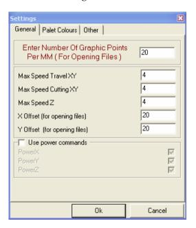
Number of Points Per MM: This is the points per MM that the drawing was designed at.
