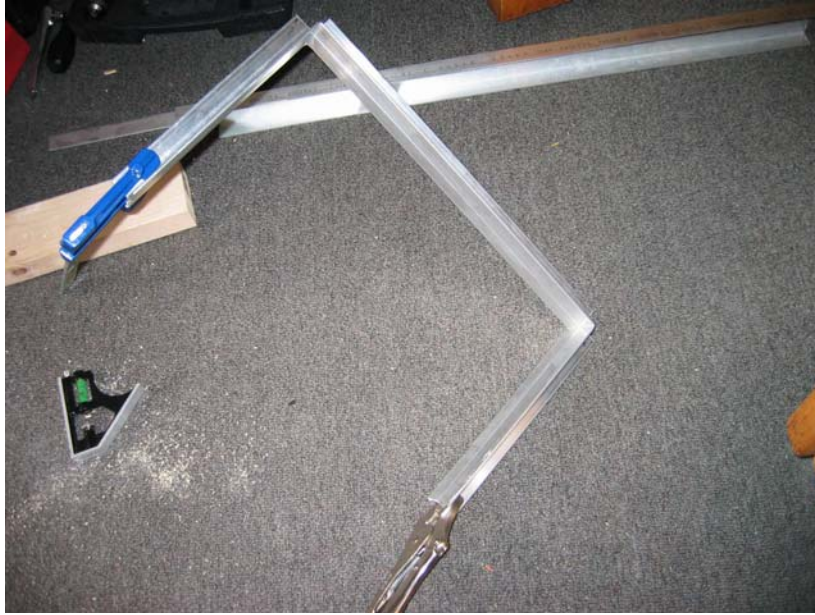
Bending both Z-axis supports at the same time to keep them identical
