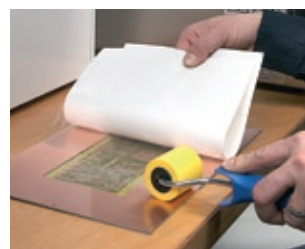
Applying the protection film
