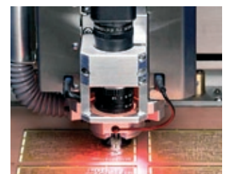
Drilling the board
