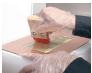
Using the squeegee to apply the paste
