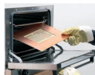
Curing the paste in a hot-air oven
