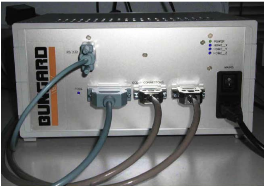
Pict. 1: ATC control unit
