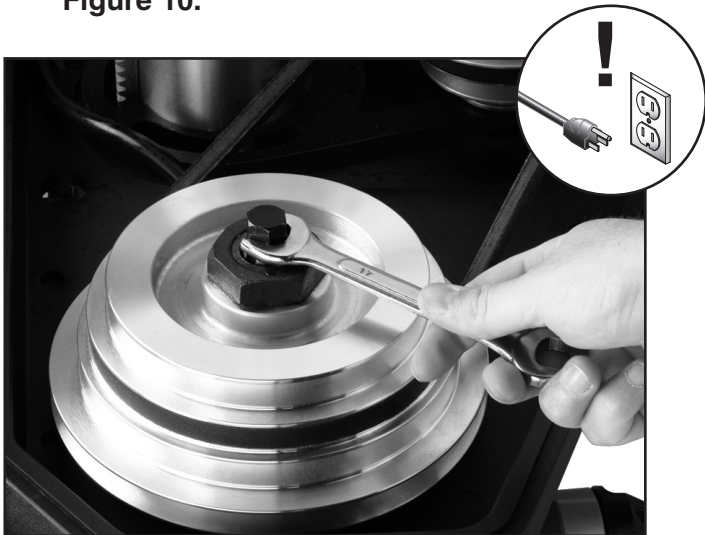
Figure 10. Turning the drawbar nut.
