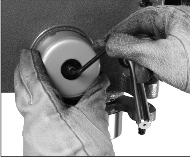
Figure 29. Loosening cover and cap screw.
