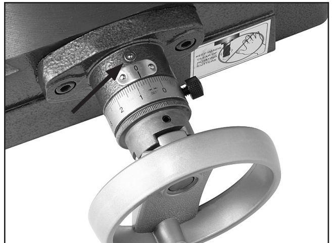
Figure 26. Handwheel oiling location.
