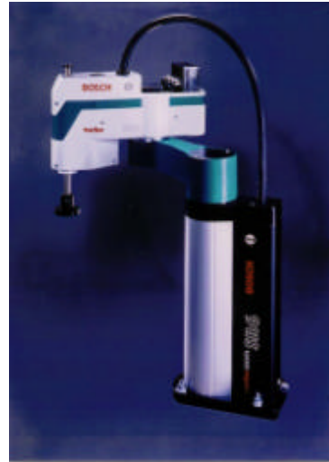
Fig. 8: SCARA Robot (Source: Bosch Rexroth AG)
