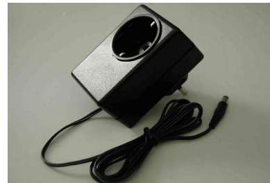
Pict. 6: Vacuum cleaner switch box
