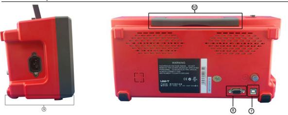
⑦ & ⑧, USB Port and RS-232 Port Combined with Digital Oscilloscope Virtual Panel for PC Connectivity
