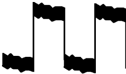
Typical peak detect display
