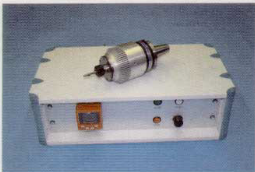
HFK 95.1 Q with automatic coupling for ATC Automatic Tool Change
