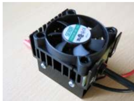
.....The condensers do fit the gap and the cooling plate freed from its plastic is glued to the cooler. The screw on the side grab behind the coolerbody's fins.
