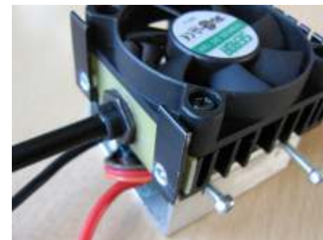
.....The condensers do fit the gap and the cooling plate freed from its plastic is glued to the cooler. The screw on the side grab behind the coolerbody's fins.
