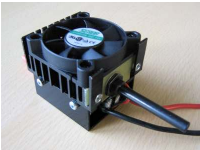
.....The condensers do fit the gap and the cooling plate freed from its plastic is glued to the cooler. The screw on the side grab behind the coolerbody's fins.
