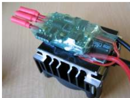
.....The condensers do fit the gap and the cooling plate freed from its plastic is glued to the cooler. The screw on the side grab behind the coolerbody's fins.
