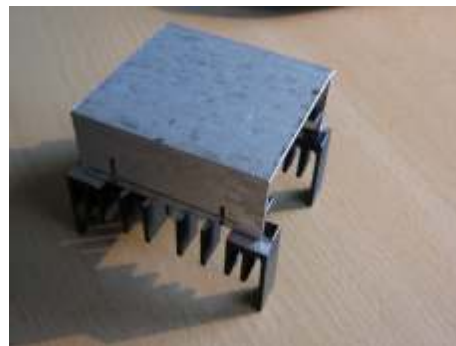
CNC - cut of course..... .....on my Bracket machine using a 5mm single side cutter .....Some scrap U shape alu profile over the cooler-block protecting the electronics
