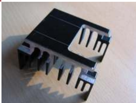
CNC - cut of course..... .....on my Bracket machine using a 5mm single side cutter .....Some scrap U shape alu profile over the cooler-block protecting the electronics
