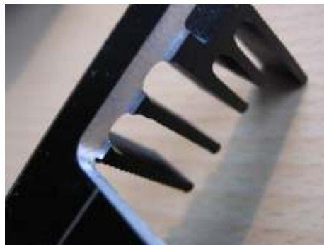
CNC - cut of course..... .....on my Bracket machine using a 5mm single side cutter .....Some scrap U shape alu profile over the cooler-block protecting the electronics
