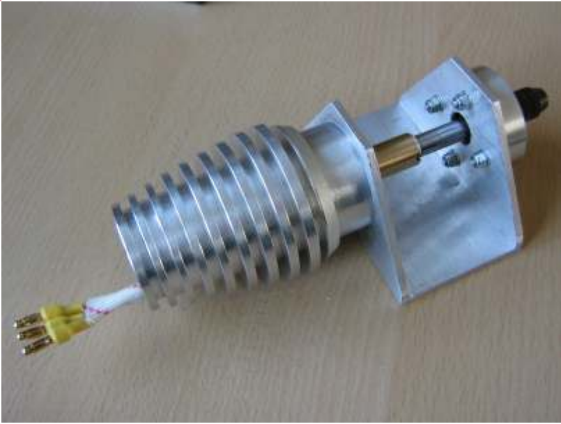
.....This is the motor mount into a cooler body cut and shaped on a lathe As this is a testrig it was convenient to mount it onto a piece of scrap U-shaped Alu. All parts are easy accesble this way.
