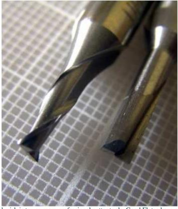
( A additional wish is to use more professional cutter tools. Good Flutes have a thicker shaft Here two cutter types with a 6mm shaft )
