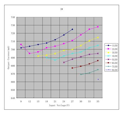
Output current corresponding to input voltage of the key points @ different number of LEDs connected in series is listed for reference in the following table.
