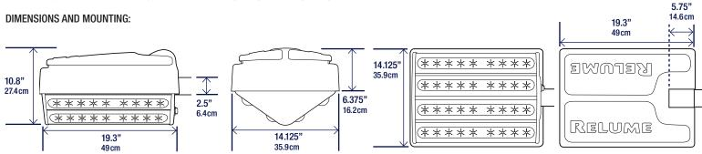
HOUSING: Aircraft Quality 6061 Aluminum is extruded to form the skeletal structure and thermal dissipation sink all in one. The unit is then capped with a TPO composite, thermo formed solar shield limiting solar heating, preventing thermal degradation of the LED LIGHT engine. A solar shield is attached with stainless steel push pin latches to provide easy tool-less access to the luminaires.
