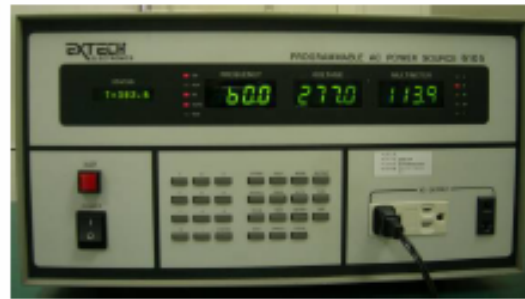
AC Power Source(277.0Vac)
