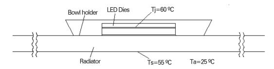
Above test data was measured by no wind conditions
