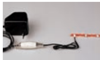
3. Connect the transformer and LED CHANNEL FLEX PCB TYPE VERTICAL together with connector.
