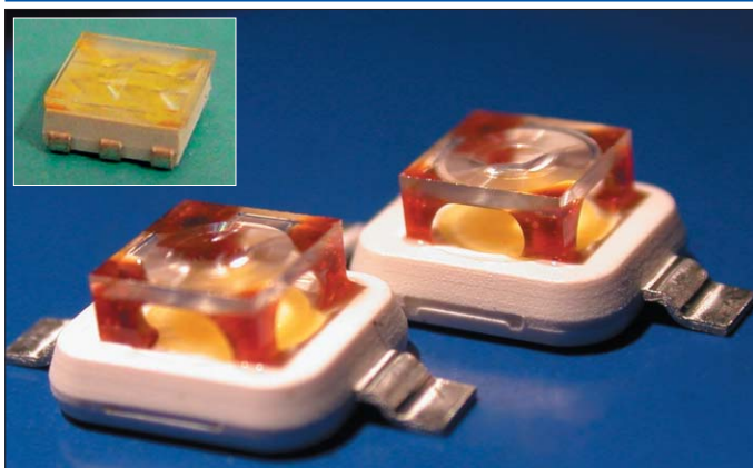
Fig. 4. Beam-shaping elements with a replicated DOE, assembled using replicated mounting pins. Inset shows latest version.
